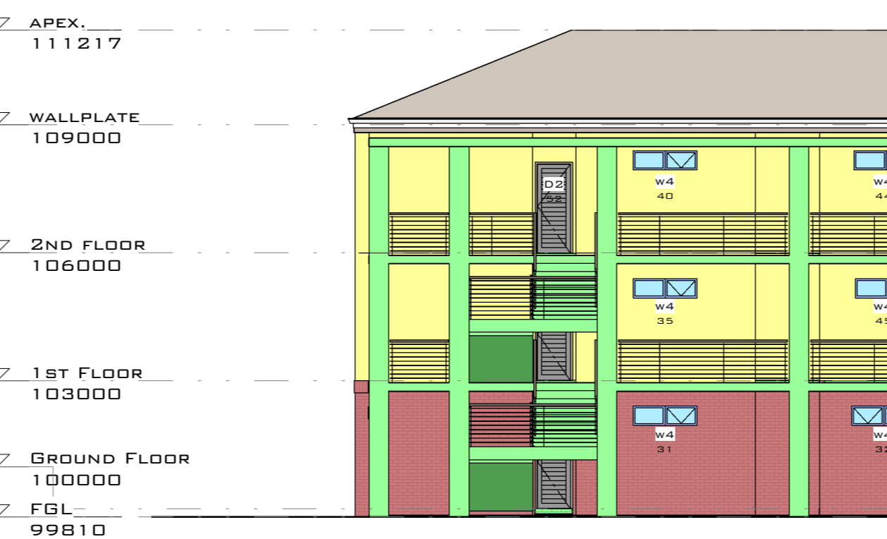
SOUTH ELEVATION SCALE: 1 : 125
